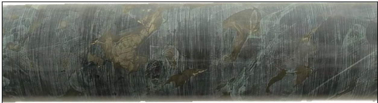
FIGURE 7.18 ORTHOCUMULATE CLINOPYROXENITE WITH CUMULATE PHASE PYRRHOTITE, PENTLANDITE AND CHALCOPYRITE FROM LAGOA DA ONÇA
