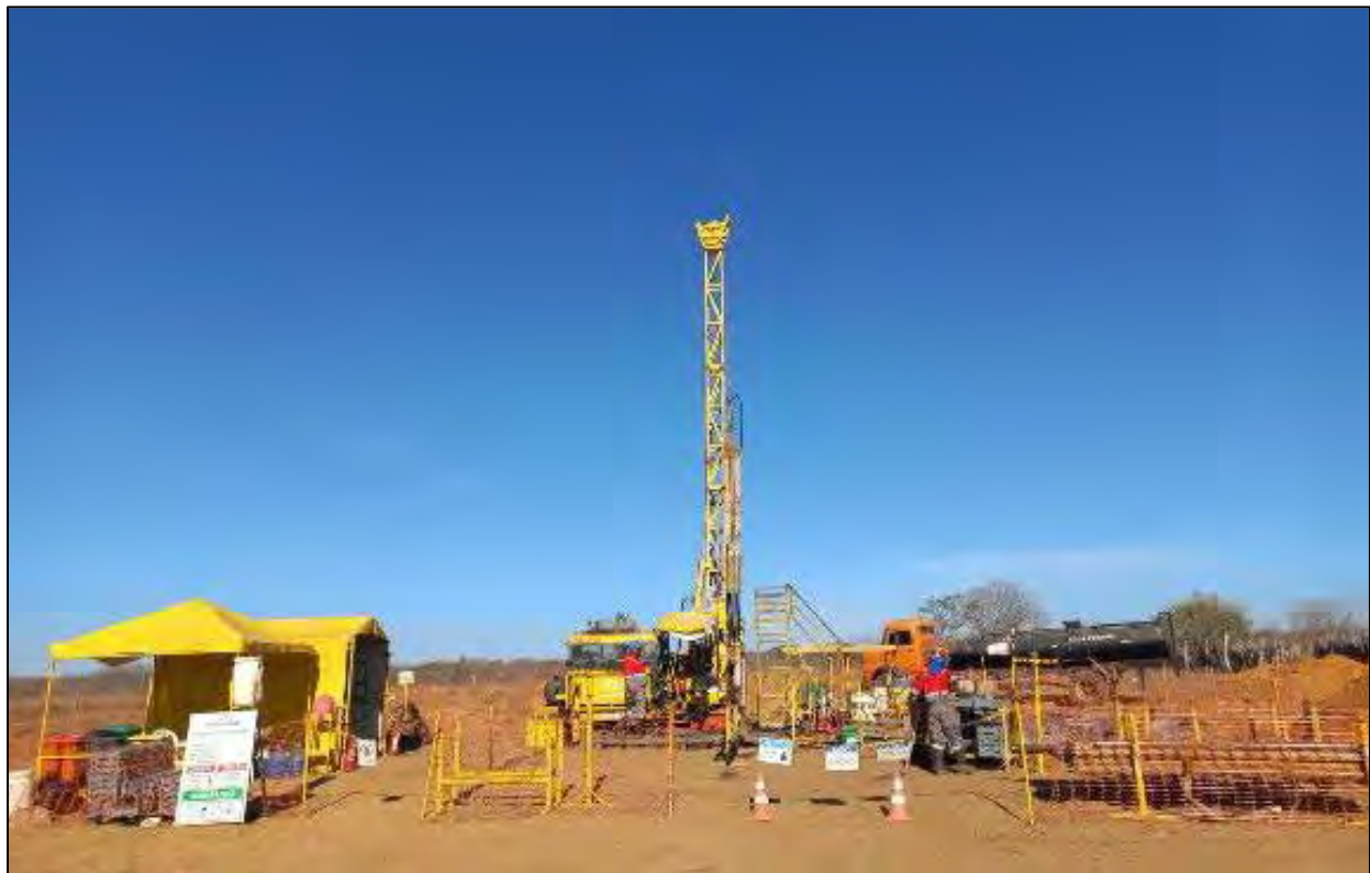
FIGURE 10.1 DIAMOND DRILL RIG SET-UP AT MANGUEIROS SITE
