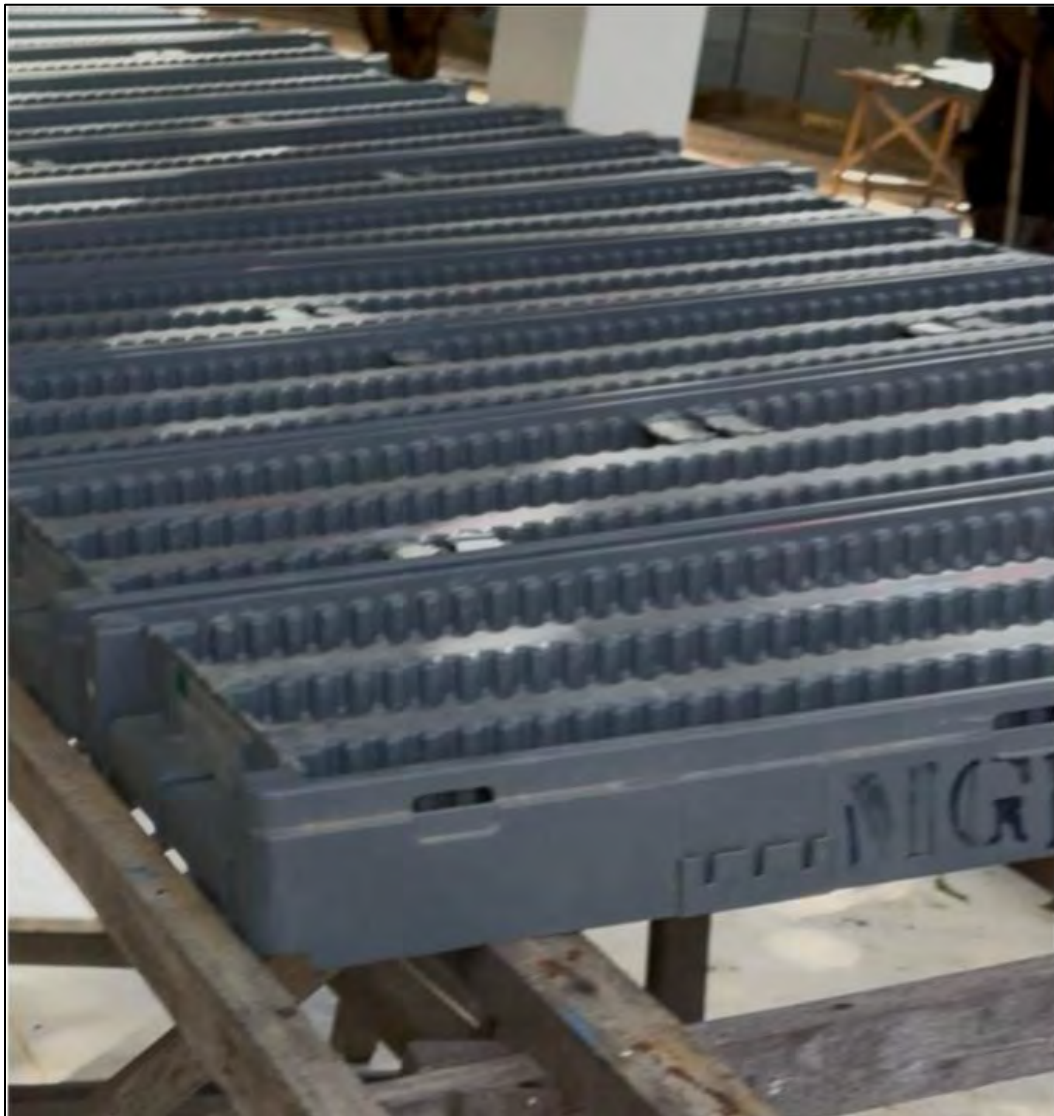
FIGURE 12.2 PLASTIC DRILL CORE BOXES USED AT MANGUEIROS
