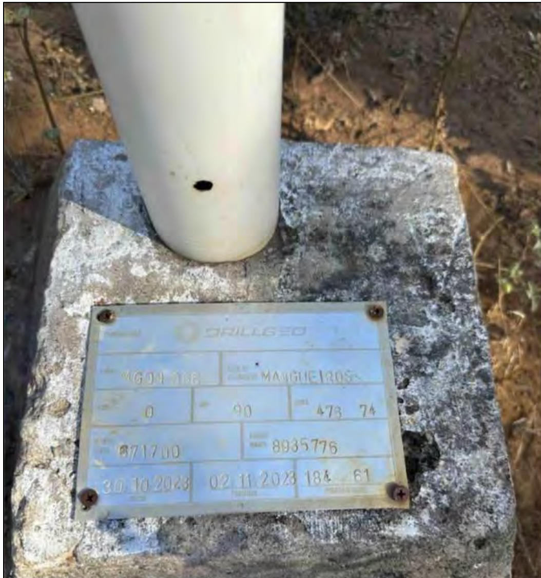
FIGURE 12.3 DRILL HOLE COLLAR MONUMENT FOR MGDH-066
