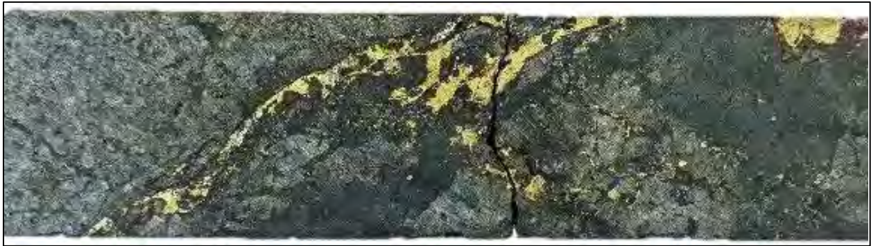
FIGURE 7.19 INTERSTITIAL CHALCOPYRITE, PYRRHOTITE, AND PENTLANDITE FROM LAGOA DA ONÇA NORTH
