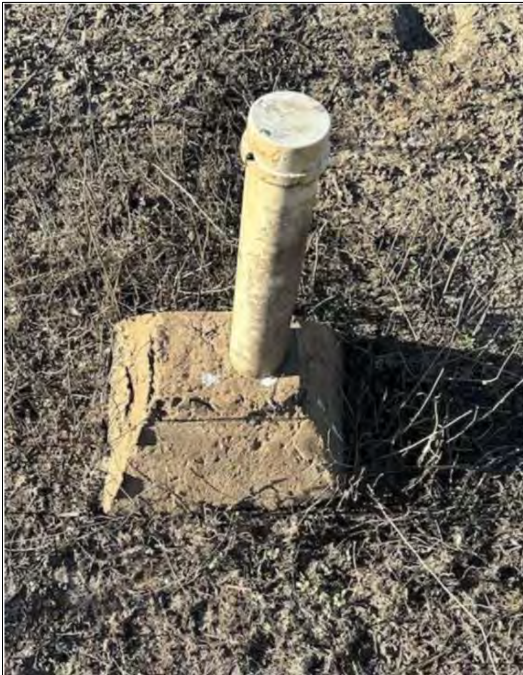
FIGURE 12.5 COLLAR MONUMENT FOR OLDER DRILL HOLE MGDH-05
